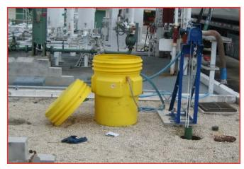
The PetroXtractors' simplicity was a great asset. After picking up the oil, the belts travel over head pulleys on each drive unit and through tandem wiper blades. Oil is then scraped off both sides of the belt and discharged through a small hose. Installation consists of merely lowering the belt and tail pulley into the casing until the pulley is fully immersed, placing the discharge hose in a container and switching the unit on.
